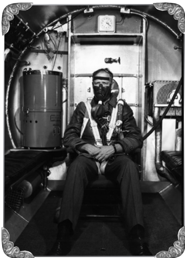
Charles A. Lindbergh, outfitted with Mayo's BLB oxygen mask, tested bail-out techniques for the P-47 pursuit aircraft in 1942.
